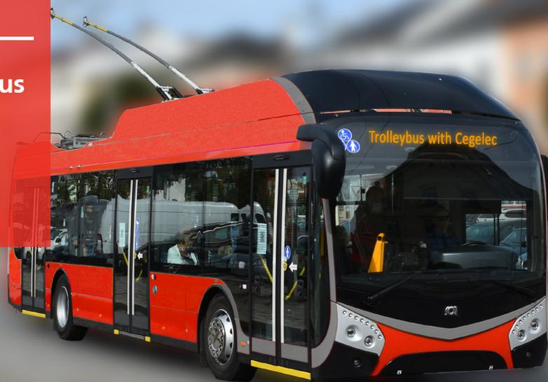
A trolleybus with dynamic charging is the best way to reduce emissions from public transport and to transition to electromobility while ensuring economical sustainability. A trolleybus equipped with traction batteries is a modern means of transport that uses overhead line in a part of its route for charging while running, eliminating unproductive vehicle downtime.
